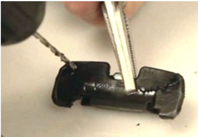
Standard Lace clip have 4 Cutting Marks and 12 holes.
